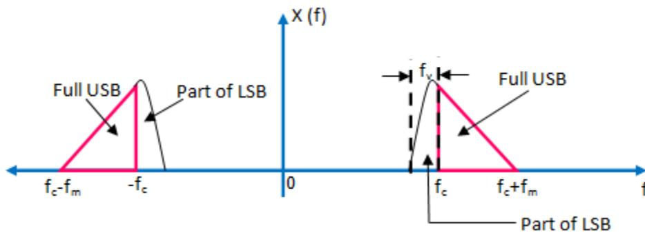
14. Consider the signal whose spectrum is as shown in Figure. Modulates the sinusoidal carrier signal of 1MHz. Draw the spectrum of DSB-SC signal and SSB-SC (upper sideband ) signal. (Nov-2014)
